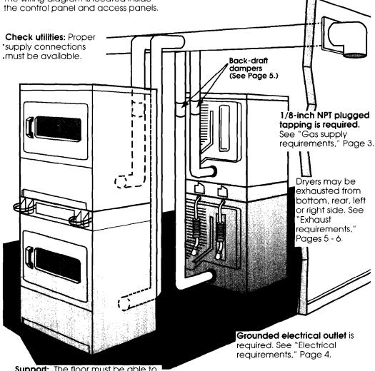
Support: The floor must be able to support the total weight of 315 pounds per unit.
